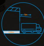
**DOCK HEIGHT:** • Doors are at 1.35m to facilitate loading. • A 5m canopy enables offloading during inclement weather.
