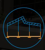
FLOORS: FM2 Large panel fibre reinforced floors 160mm thick 35Mpa, UDL of 80KN per m².
